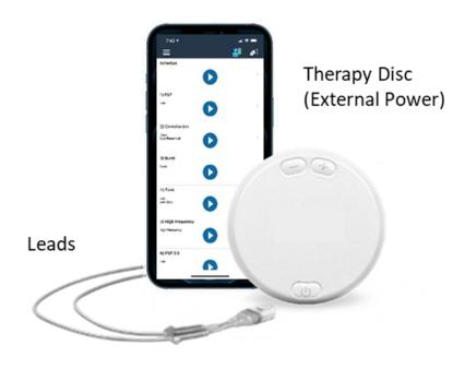
Battery-free, micro-Implantable Pulse Generator (mIPG)
